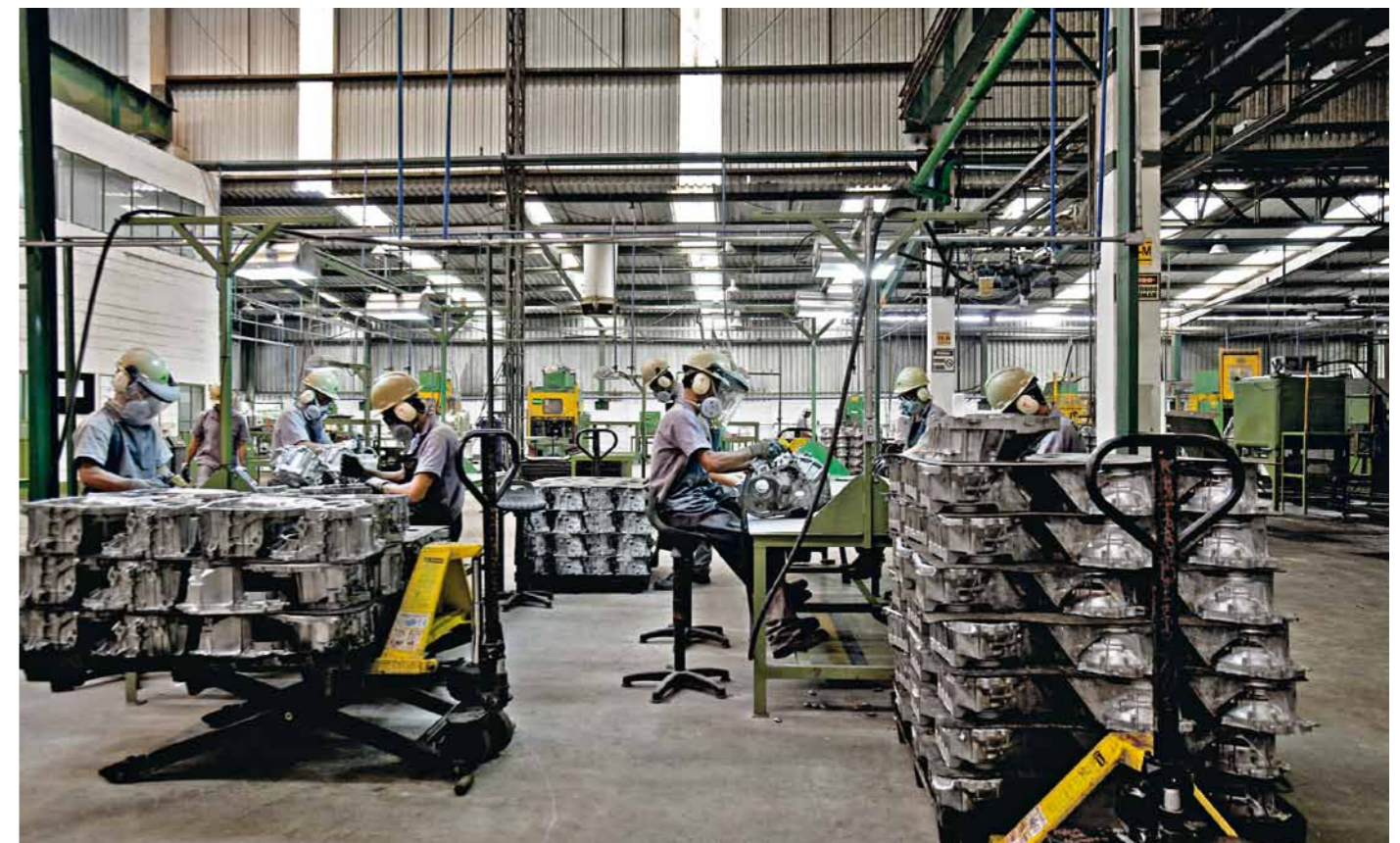
Cast and polished: Rima turns the metal into engine mounts and transmission housing for ultra-light automobiles.
