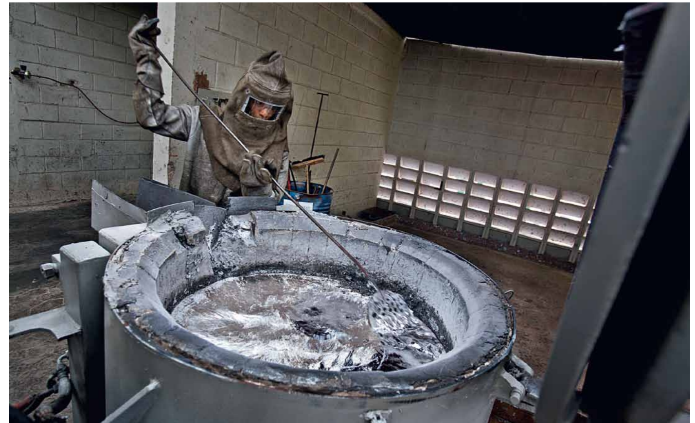
Intelligent processes. Once rendered, the molten metal is not poured into bar moulds but into vats, which are rolled directly into production.
