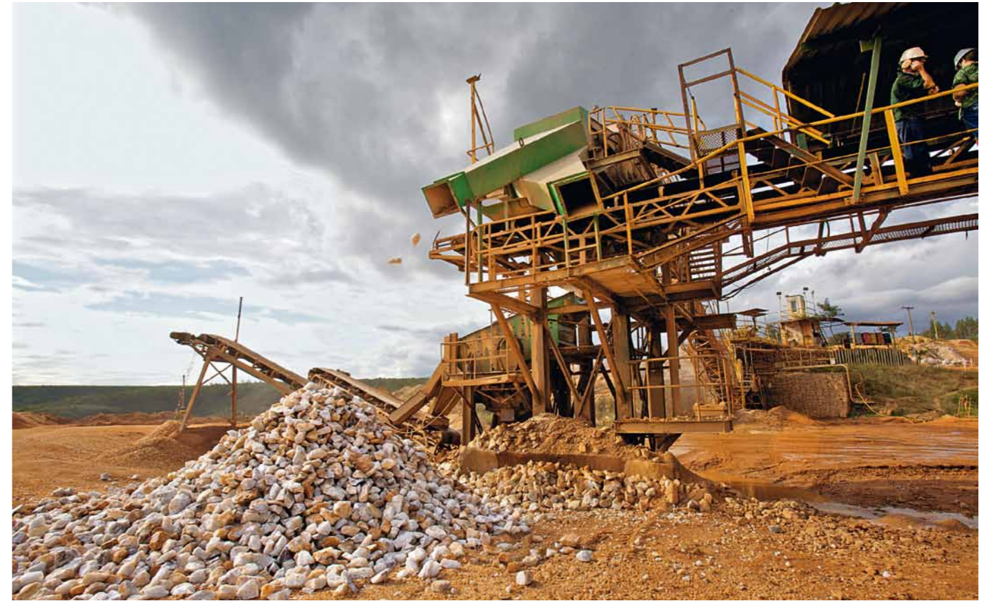
A tough business: The stone mill crushes the shimmering white quartz, which is then loaded into the blast furnaces.
