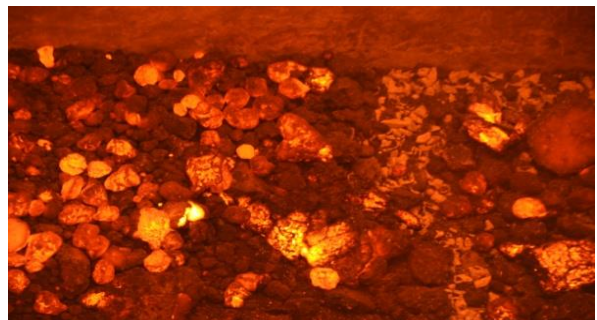
Raw materials being burned to clinker
